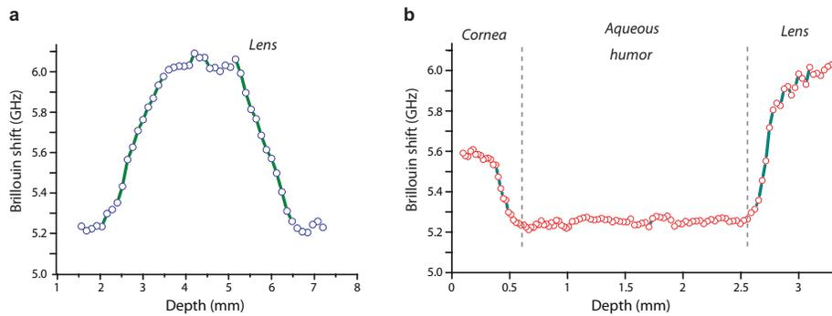
Fig. 4. *In vivo* Brillouin measurement of a human eye. (a) Depth profile of the crystalline lens. (b) Depth profile of the anterior chamber. The data are an average of four such scans taken ten minutes apart.
